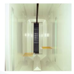
Automated coating of complex parts with reciprocators and base movers.
