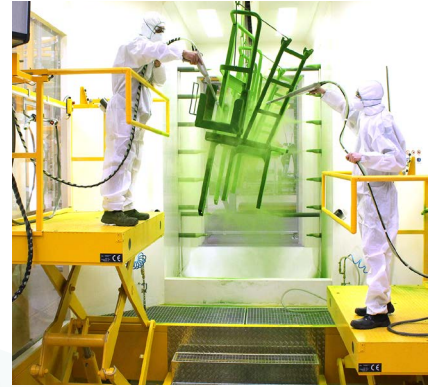
Flexible powder coating of flat and / or large workpieces.
