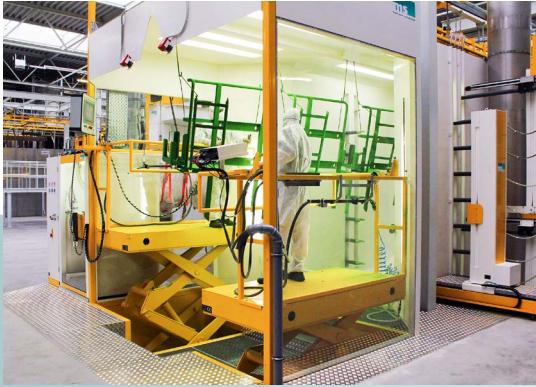
Manual coating area with integrated scissor lift tables.
